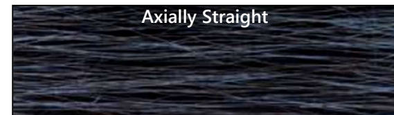
Carbonized PAN filaments (Lee, 1998)
