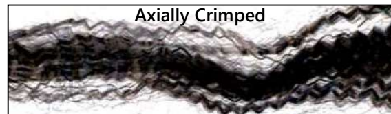
Carbonized rayon filaments (Lee, 1998)
