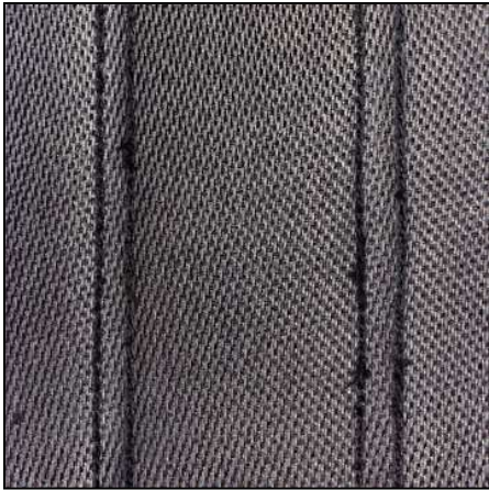
Machine stitched lay-up (Lee, 1987)
