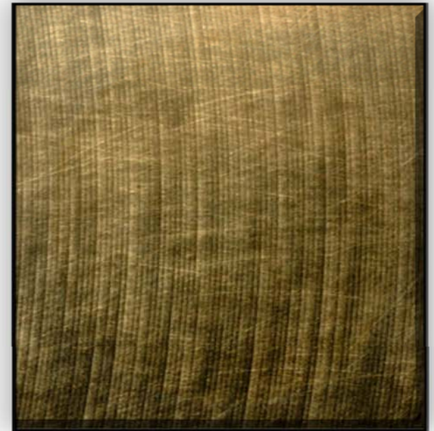
Titanium 64 in Pretreat – Starting potential was -0.75 V; no signs of any damage to the oxide or base metal were observed
