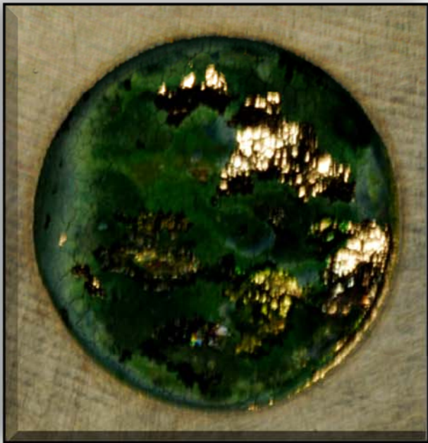
Inconel 625 in Pretreat – Starting potential was -0.5 V; significant etching (recession), hydroxide formation and possible plate-back of liberated Cr atoms onto base metal surface
