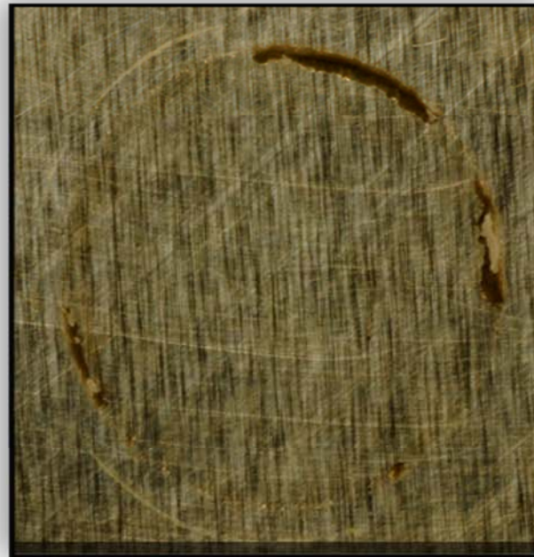
Cronidur 30 in Pretreat – Starting potential was -0.75 V; other than some apparent crevicing near the o-ring, no etching, recession or large-scale oxide destruction was observed
