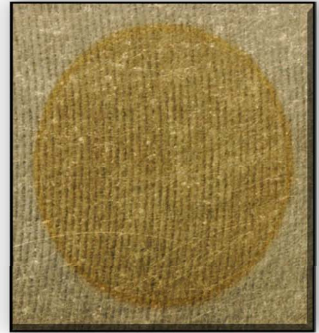
Titanium CP in Pretreat – E_{Ver} was 4.2 V; appearance typical of most Ti samples; no base metal damage on any of the Ti samples even when subjected to higher voltage
