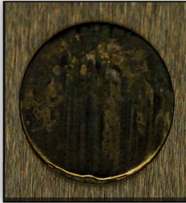
Inconel 625 in Brine – E_{Ver} was 4.5 V; general etching into base metal (loss of oxide, loss of base metal); similar to the stripping effects noted in other peculiar test runs (next topic)
