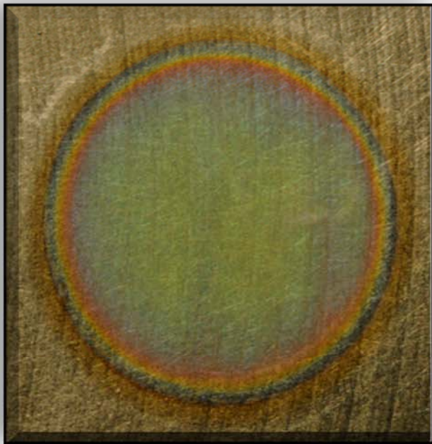
Titanium LI in Pretreat – No unusual test conditions or results were noted; E_{Ver} was 2.2V; atypical in appearance (oxide aberrations)
