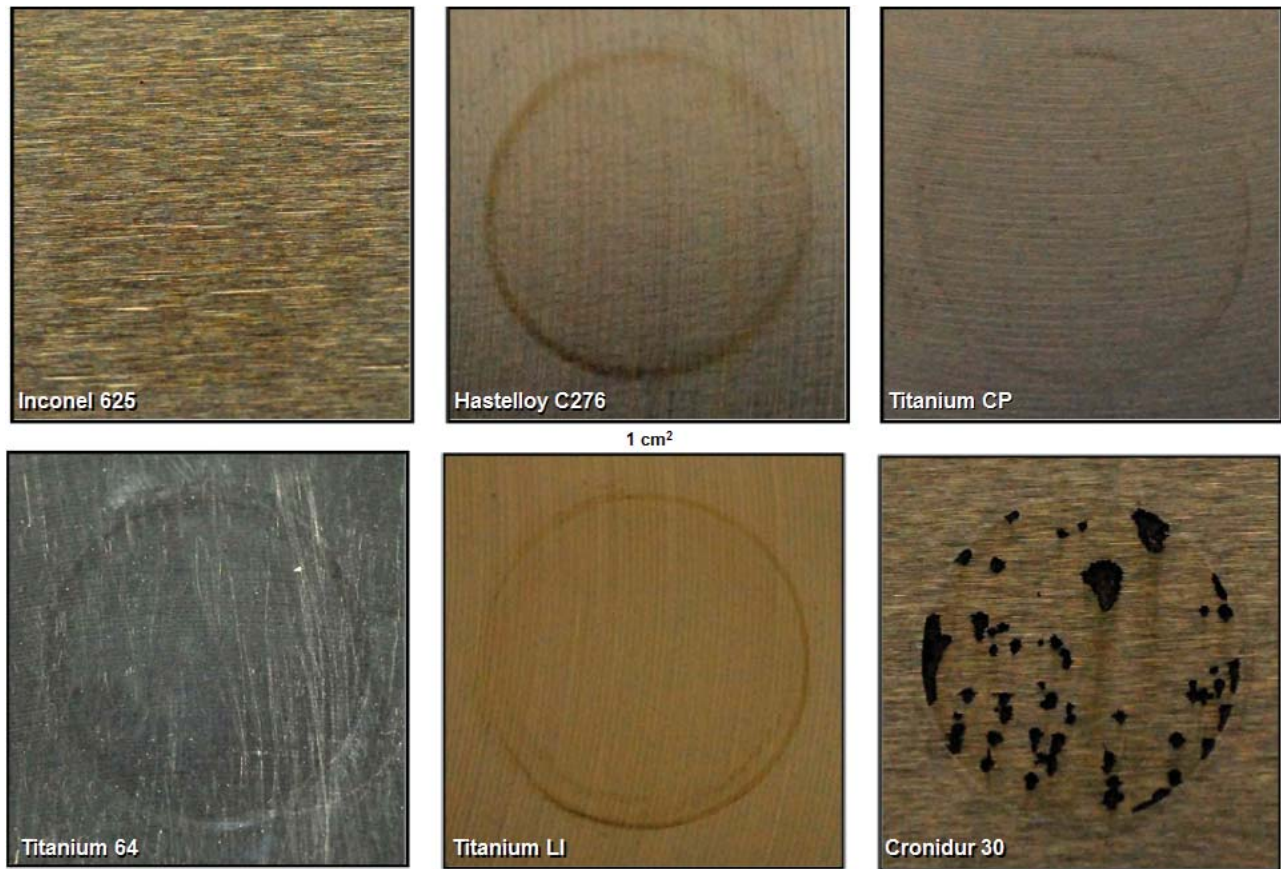
Figure 7: Photographs of some of the test areas for the six metals after cyclic polarization in brine solution.
