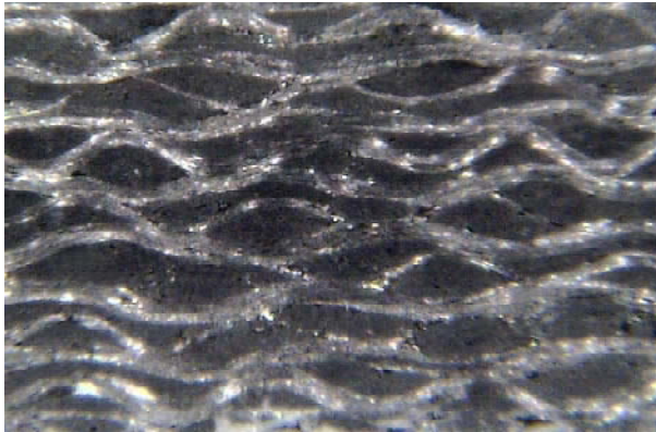
Cross-sectional thickness image of carbonized rayon fabric-reinforced / charred phenolic-matrix laminate
